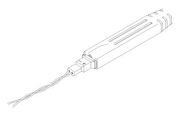
Figure 5: Twisting the Input Leads
