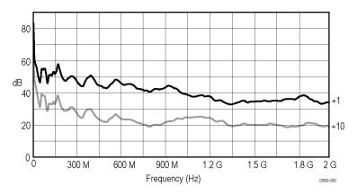
Figure 6: Typical Common-Mode Rejection Ratio (+1 and +10 attenuation)
