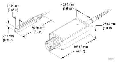
Figure 8: Probe head and compensation box dimensions
