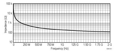
Figure 7: Typical differential input impedance versus frequency
